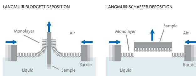
FIGURE 1: ILLUSTRATIONS OF LANGMUIR-BLODGETT AND LANGMUIR-SCHAEFER DEPOSITION
