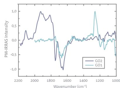
FIGURE 3: GRAPHENE CHARACTERIZATION. PM-IRRAS was used together with a Langmuir trough to measure two different types of floating graphene oxide layers prepared on a water subphase. The C=O stretches of the two layers oriented differently ( $1750 \text{ cm}^{-1}$ ) in the floating layer. The spectra shows that  $\text{GO}_2$  has much more complex structure, probably from having more defects in the graphene layer.
