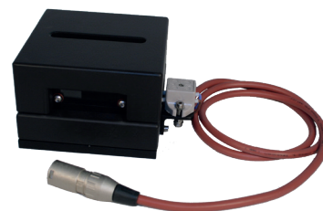
Measuring chamber, electrically heated (C203E)
