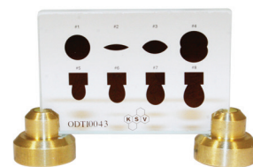
Contact angle and surface calibration pack (C216A)
